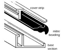
**HELPFUL HINTS** - To achieve a neat mitre, insert a small piece of mitre beading between the base and cover strip at the point where the mitre is to be cut. Cut the mitre through all sections. This beading has the effect of holding the cover strip at the correct angle so that when applied to the sheet it results in a neat mitre.
