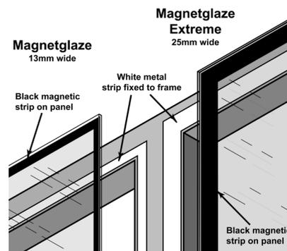
**HELPFUL HINTS** - For larger windows (1200mm x 1200mm or bigger) we strongly recommend placing a couple of screws under the glazing panel to support the sheet. This will remove the risk of the sheet slipping down and becoming detached. Alternatively, consider using new Magnetglaze Extreme.
